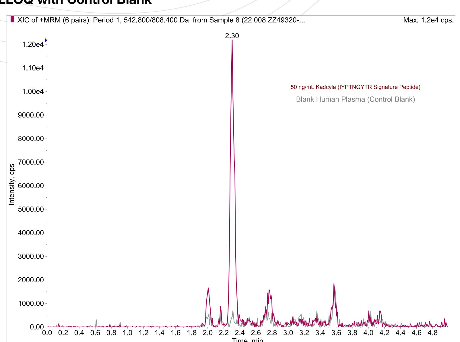
Figure 3 shows the chromatogram highlighting the retention time (2.30 min) and peak height of signature peptide (IYPTNGYTR) monitored at a lower limit of quantitation (50 ng/mL). The chromatogram of the signature peptide (burgundy) is overlaid with control blank human plasma sample (gray).
