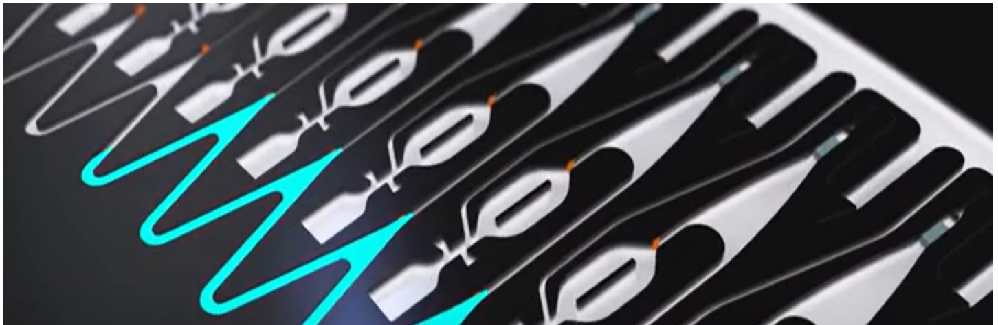
Figure 1: Gyrolab microfluidic disk in detail: Capillary action and centrifugal force deliver the reagents and samples to a nanocolumn.
