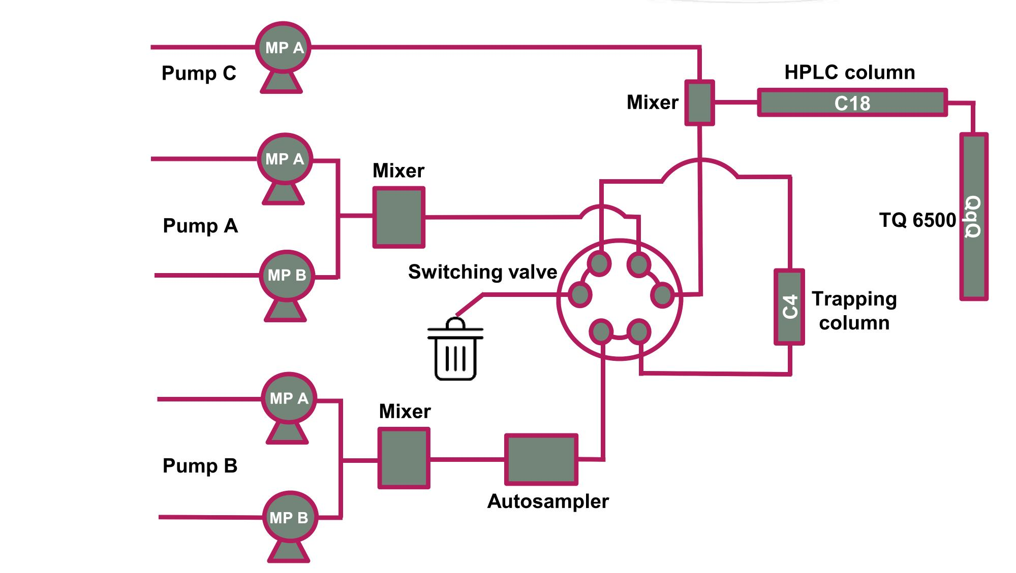
Figure 2: Schematic representation of the chromatographic trap-and-elute system (loading position).
