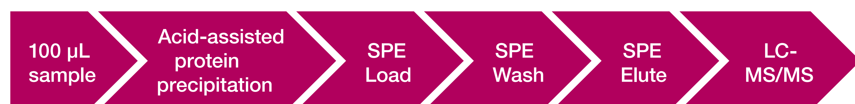
Figure 1. Sample extraction procedure from human serum and surrogate matrix.
